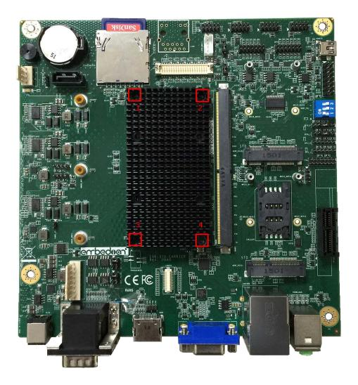
5. Use 4 units of M2.5 12mm sized screws to affix the heatsink together with the system.
