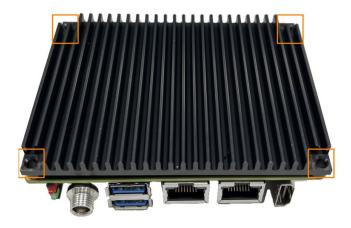
$4. \quad \text{Use 4 units of M3 sized screws to affix the heatsink together with the system}.$
