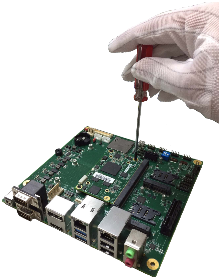
Figure 14: Fasten SMARC Module
