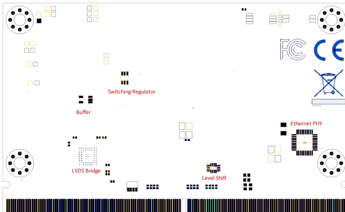
Figure 18. SMARC-iMX8M Bottom Side Components
